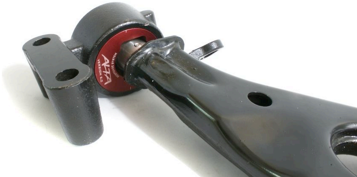
Control arm installed into PSRS
